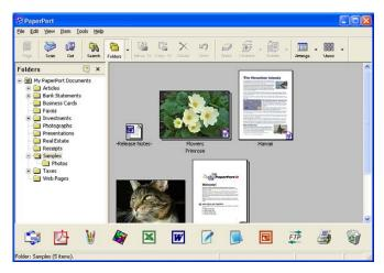
**Page View** displays a close-up of a single page and you can open a PaperPort<sup>®</sup> SE item by double-clicking it. As long as you have the proper application on your PC to display it, you can also double-click a non-PaperPort<sup>®</sup> SE item to open it.
